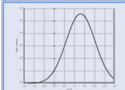
**Figure:** Pore size distribution by Inverse GPC, data evaluated with PSS PoroCheck software. PSS SUPREMA column set.
