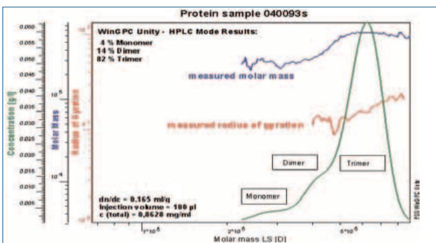
**Fig:** Mono-, Di- and Trimer Protein Aggregates tested with SLD 7000 MALLS Detector and WinGPC Unity Light Scattering Module
