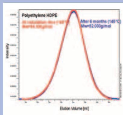
Six Months stability of a PSS POLEFIN column set. (GPC testing of broad High Density Polyethylene Standard).
