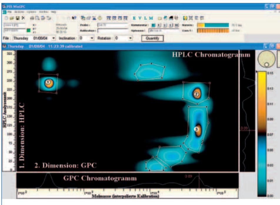
**Figure:** WinGPC Unity 2D chromatography module: GPC separation only: coelution of Peak 2 and 3; HPLC separation only: peak 1 and 2 not separated. With 2D: all peaks are well resolved
