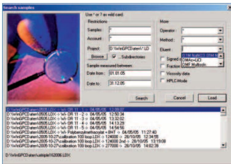
Statistic for all samples analyzed in 2005. The field „Eluent“ shows all eluents that have been used during that period. If an eluent is selected, WinGPC shows the number of samples and the sample information of all samples measured in 2005 with this eluent.
