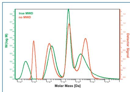
Fig. 2: Overlay of a real (green) with a molar mass distribution (red), wrong calculated by a HPLC data system
