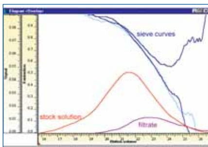
Fig. 1: Overlay of stock solution and filtrate (only one) GPC/SEC chromatograms. The resulting sieve curves for all three UF membranes for water treatment are displayed too
