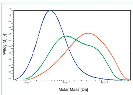
**Fig. 1:** Separation of Amylopectin, Amylose and potato starch on PSS GRAM columns (30 000 Å 10 µm 8 x 300 mm + precolumn). Conditions: eluent: DMSO, LiBr 5 g/l; temperature: 60° C, flow rate: 0.5 ml/min; concentration: 0.5 g/l
