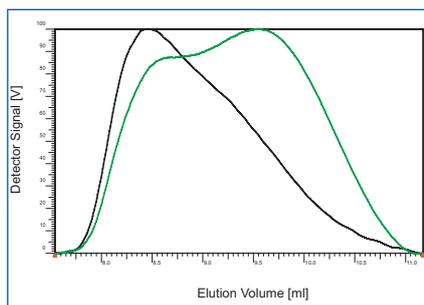
**Fig. 2:** Analysis of potato starch with RI detection (green curve) and 90° light scattering detection (black curve)
