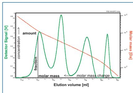
Fig. 1: GPC/SEC chromatogram of a sample mixture (green) with overlaid calibration curve (red)
