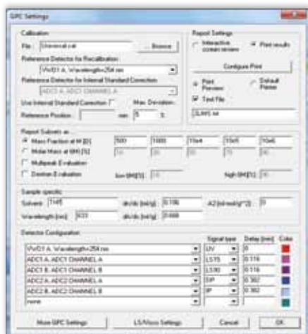
GPC/SEC data evaluation settings support up to 6 signals and conventional, LS, DV and triple detection systems
