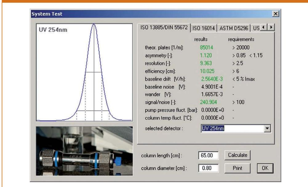
Alternatively, suitable test materials for a variety of typical GPC/SEC solvents are presented in Table 1. For these materials an injection volume of 20 µL (or if possible less) can be used, whereas concentration should be adapted to the number of columns used: One column = 0.2 g/L; two columns = 0.5 g/L; three columns = 1 g/L. As mentioned before, it is important to use the same test substance with the same instrument and analytical conditions for all tests.
