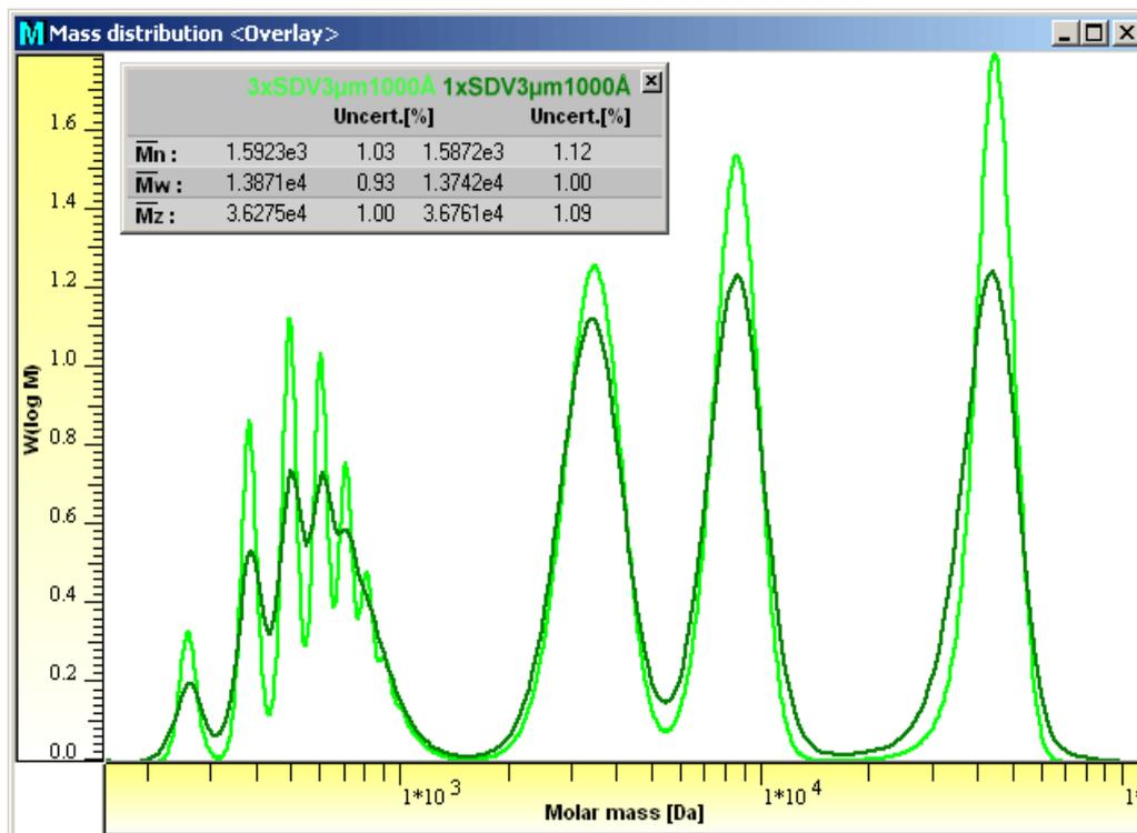
Figure 5: Influence of the number of columns on separations using SDV columns filled with 3 $\mu$ m particle size in THF. Here the results are shown for a combination of three columns (light green) compared to the results obtained with one analytical column (dark green).
